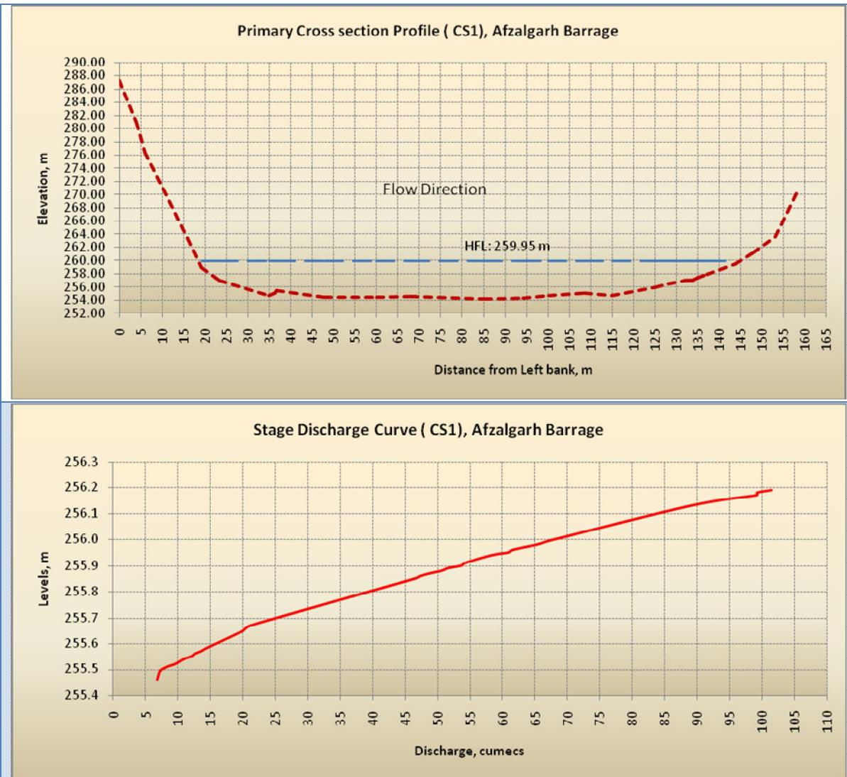
**Table 4: Hydraulic properties of Afzalgarh Barrage site (CS1)**
